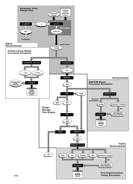
Figure A-1 Cadence/Verilog Interface Design Flow
