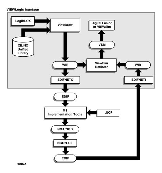
Figure E-1 Viewlogic/Xilinx Software Design Flow
