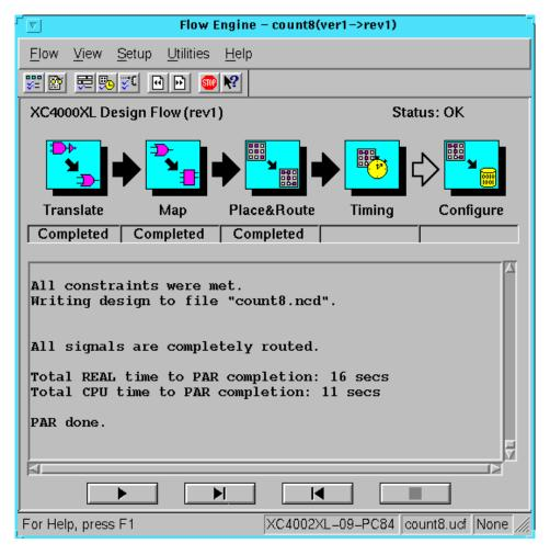
Figure 3-9 Placing and Routing Design
