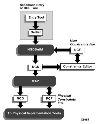
Figure H-1 Entering Design Constraints
