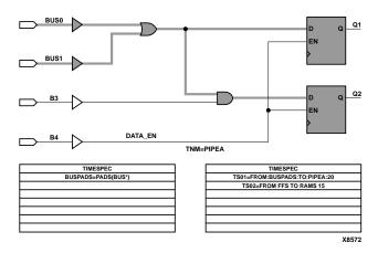
Figure H-4 Example TNM, TIMESPEC, and TIMEGRP
