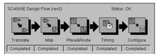
Figure 4-4 Flow Engine Design Steps
