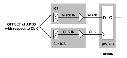
Figure H-3 Using OFFSET Constraints
