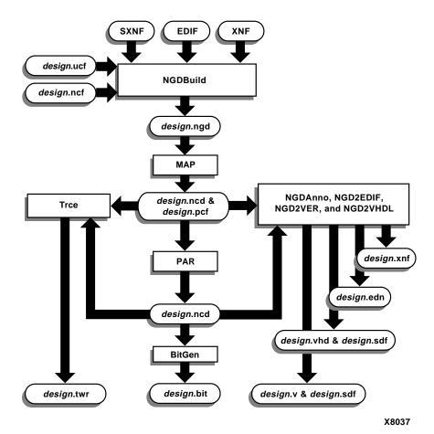
Figure 4-2 Detailed Design Flow
