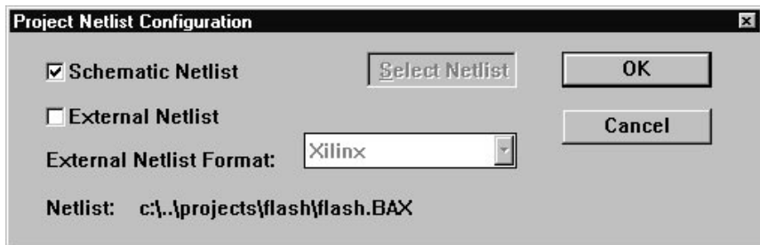
Figure 1-20. Selecting A Netlist For Simulation.
