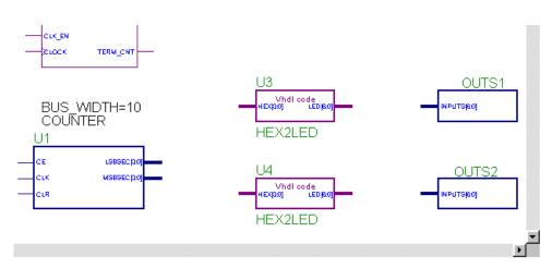
Figure 1-26 Placing the HEX2LED Component
