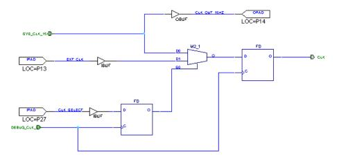
Figure 6-5 Clock Muxing Circuitry
