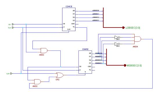
Figure 1-11 Completed CNT60 Schematic
