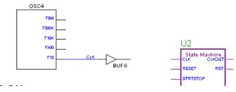
Figure 1-34 Placing the BUFG
