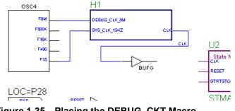
Figure 1-35 Placing the DEBUG\_CKT Macro
