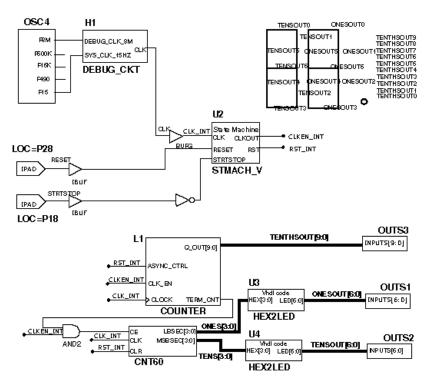
Figure 1-36 Completed Watch Schematic
