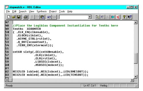
Figure 2-12 Verilog Component Instantiation of LogiBLOX Module
