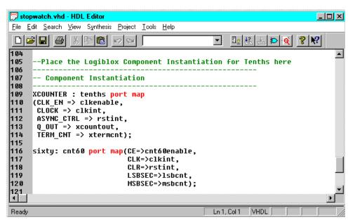
Figure 2-10 VHDL Component Instantiation of LogiBLOX Module
