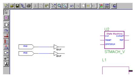
Figure 1-28 Placing RESET and STRTSTOP I/O Components
