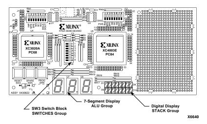
Figure 6-1 FPGA Demonstration Board Components
