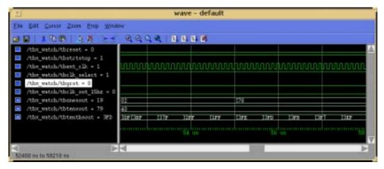
Figure 1-4 Simulation Output in Wave Window
